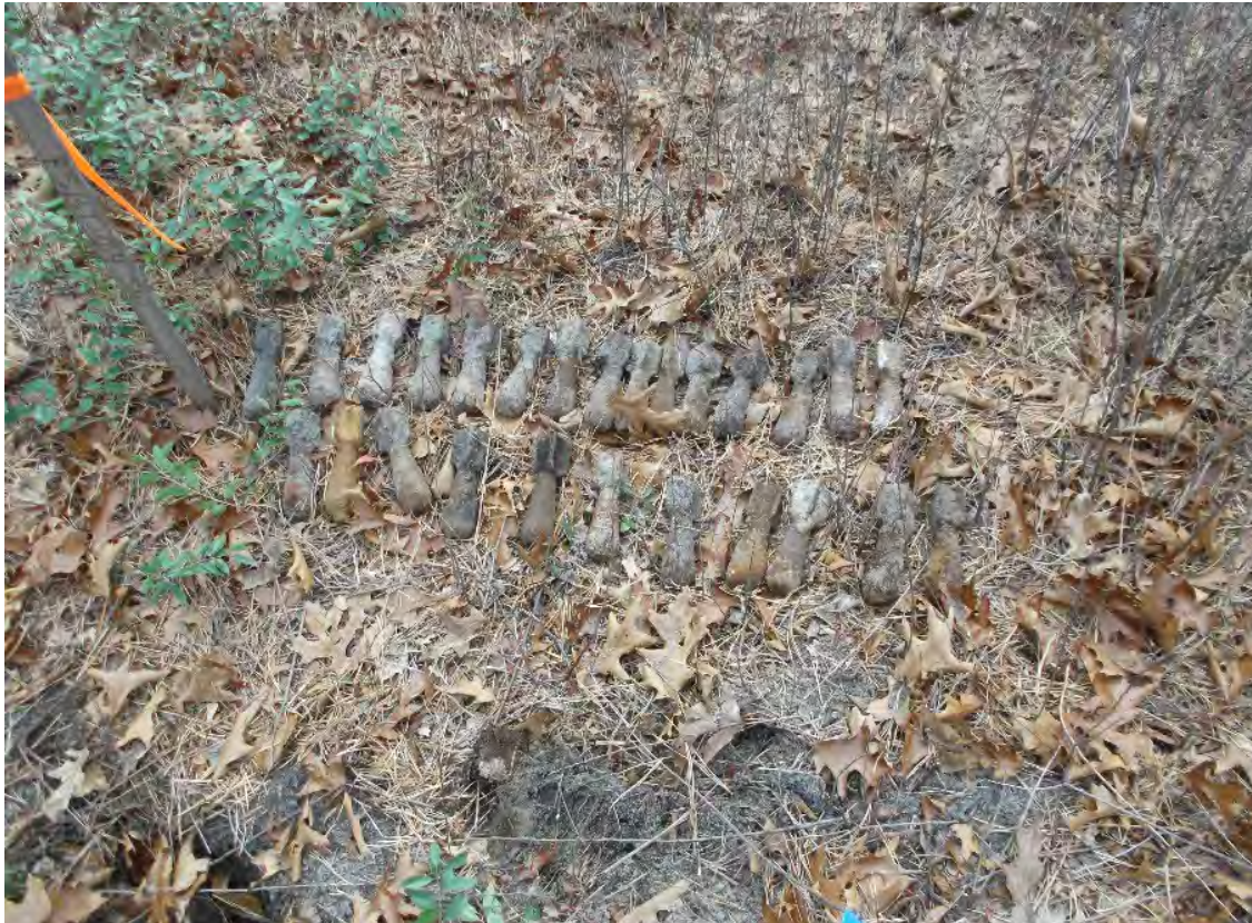
Recovered MEC (MK23 3-lb Practice Bombs and MK5 Practice Bombs with MK4 Signal Cartridges)
